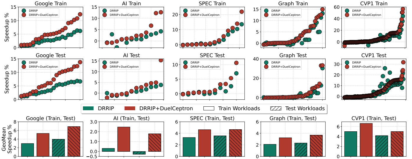
Fig. 5: Performance of DRRIP and DRRIP+DuelCeptron across the train set and test set of workloads.
