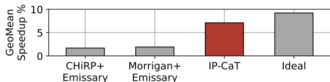
Fig. 1: Comparison of IP-CaT with i) combinations of the state-of-the-art TLB replacement policy (CHIrp [5]), instruction TLB prefetcher (Morrigan [4]), and code-aware cache replacement policy (Emissary [6]) and ii) an idealized upper bound combining optimized TLB and cache management for L1I prefetches. This comparison considers EPI as L1I prefetcher [1] and 105 server workloads.
